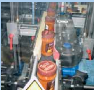
Motorized wrapping unit for smoothing.
